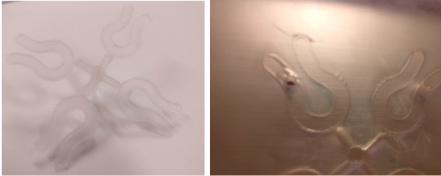
Fig. 6. (a) The MUD setup could produce over twenty components. (b) Fractures began to emerge at the ends of cavities.
