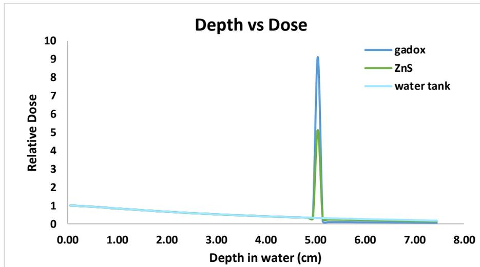
Figure 7. Depth-dose curve for the 1 mm cube gadax, ZnS and water phantoms.
