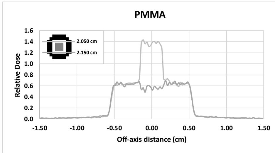
Figure 5. x-axis dose profiles taken at the depths of the PMMA layers just above and below the gadox core.
