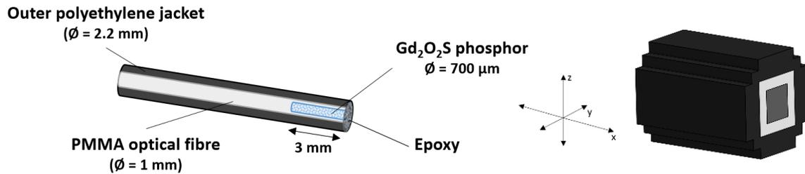
Figure 2. Schematic of the gadox-based detector<sup>14</sup> (left) and a 3-D representation of the virtual sensing tip model created in DOSXYZnrc (right).
