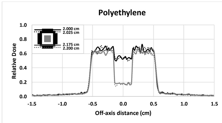
Figure 6. x-axis dose profiles taken at the four depths containing polyethylene – two entrance layers above and two exit layers below the PMMA core.
