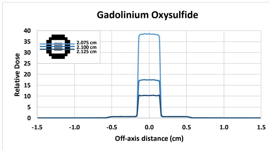
Figure 4. x-axis dose profiles taken at each of the three layers of the detector phantom containing the gadox core.
