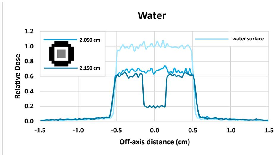
Figure 3. x-axis dose profiles taken at depths containing only water – at the surface, just above and just below the simulated sensing tip model volume.
