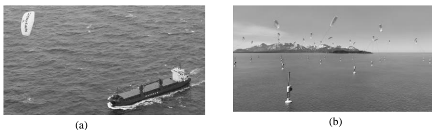
Fig. 5. SkySails productions, (a) Ship propulsion system, (b) airborne power generator (Fritz 2013)
