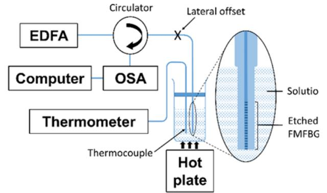
Fig. 2. Experimental setup used for sensor data acquisition. EDFA: Erbium doped fibre amplifier, OSA: Optical spectrum
