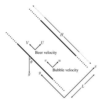
FIG. 1. Geometry of the tilted cylinder showing the coordinate system embedded in the cylinder and the components of the velocity fields of bubbles and beer. Note that the tilt has been exaggerated in this diagram.
