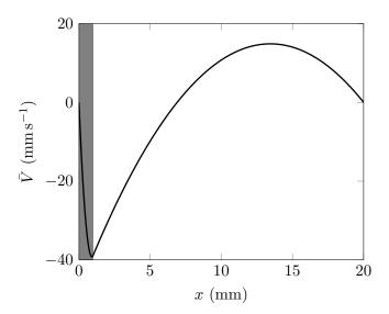
FIG. 3. Velocity in the y direction as a function of position in the x direction for the case in which  $x_1 = L/20$ . The shaded region shows the layer of pure beer. As can be seen the velocity is negative in the bubbly beer region, i.e. sinking bubbles are predicted.
