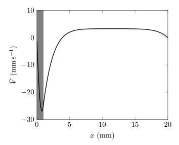
FIG. 4. Numerical calculation of velocity in the y direction as a function of position in the x direction. The bubble free region is shaded in grey.
