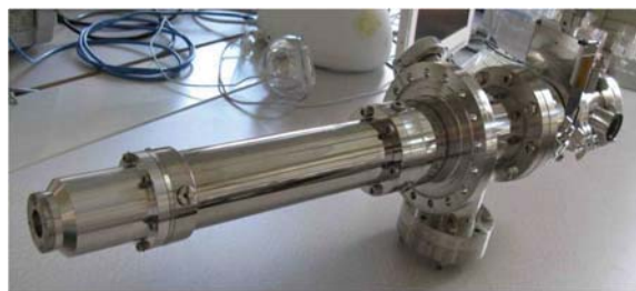
Fig. 10. Differential pumping system for the liquid jet injector. It consists of two parts, the catcher shroud and the nozzle shroud, which can be decoupled and retracted via a bayonet coupling. This allows the use of fixed samples without breaking the vacuum.
