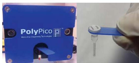
Fig. 7. (left) PolyPico dispensing head and (right) dispensing cartridge.
