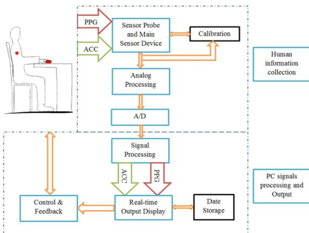
Fig 2. System Layout for Cloud Based Optical Sensor for PPG Signal Monitoring
