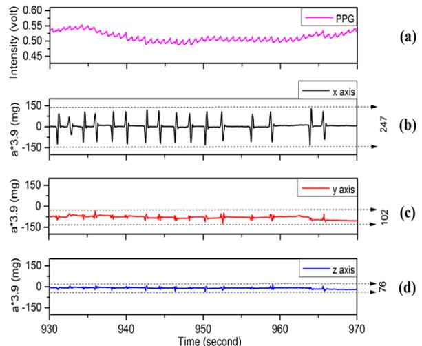
Fig 3. Real Time Data from Optical (PPG) sensor and co-located three axis accelerometer
