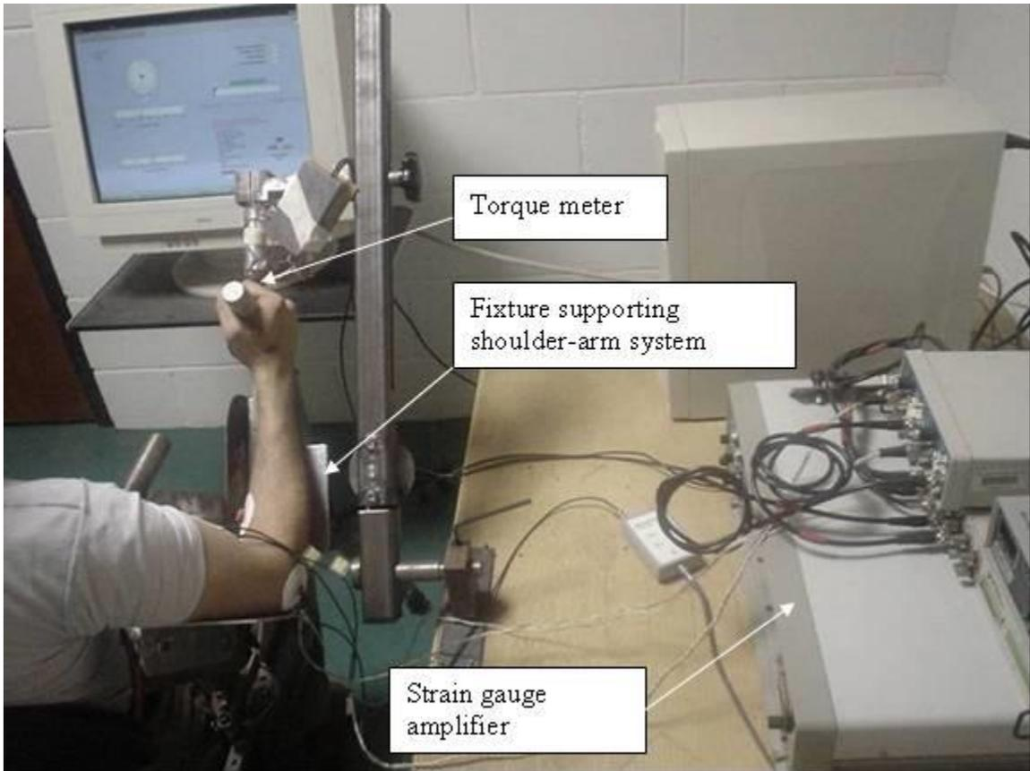
Figure 1 Fixture for keeping the shoulder arm system in position
