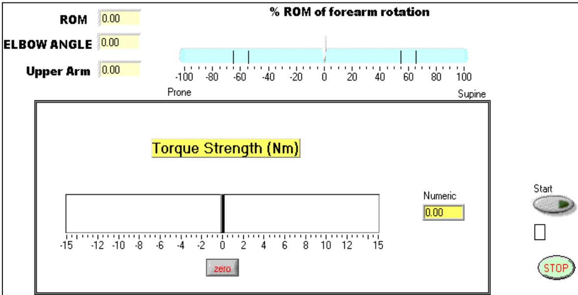
Figure 2 Screen shot of LabVIEW Virtual Instrument (VI) for recording torque
