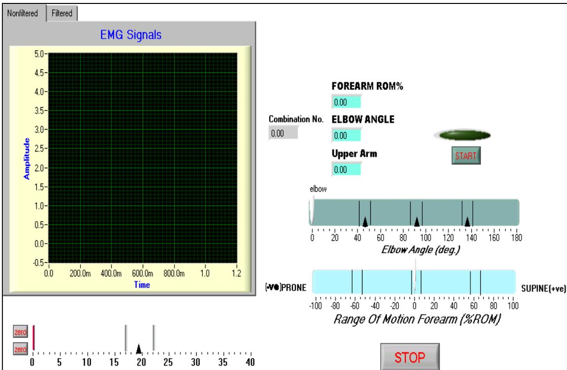
Figure 3 Screen shot of LabVIEW VI for EMG recording
