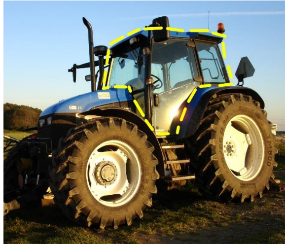
Figure 1. Typical ROPS structure (yellow dashed outline) of a modern tractor (photo from: Solitude [CC BY-SA 2.0 ( http://creativecommons.org/licenses/by-sa/2.0 )], via Wikimedia Commons).
