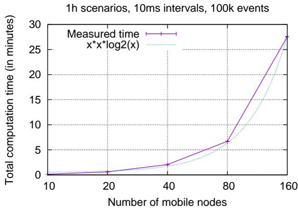
**Figure 5: Computation complexity of the discrete event processor.**
