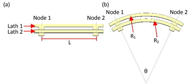
Figure 5: Relative sliding of layers, (a) as a flat grid, and (b) after deforming.
