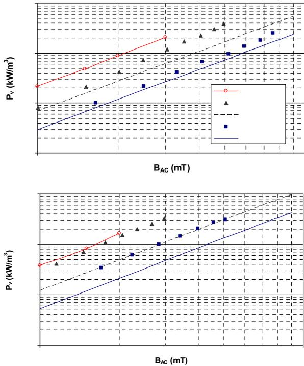
Fig. 5 Power loss density,  $P_v$ , vs.  $B_{AC}$  for metal alloys at (a) 3 MHz and (b) 5 MHz
