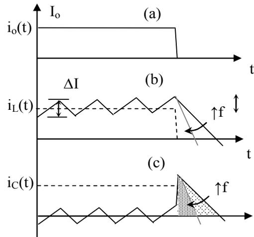
Fig. 1 POL waveforms (a) output current,  $i_o(t)$ , (b) inductor current,  $i_L(t)$  and (c) capacitor current,  $i_C(t)$
