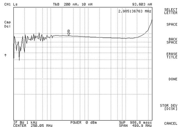
Fig. 9 Measured inductance vs. frequency for test inductor
