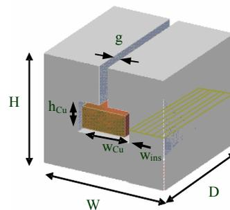
Fig. 7 Bead inductor structure
