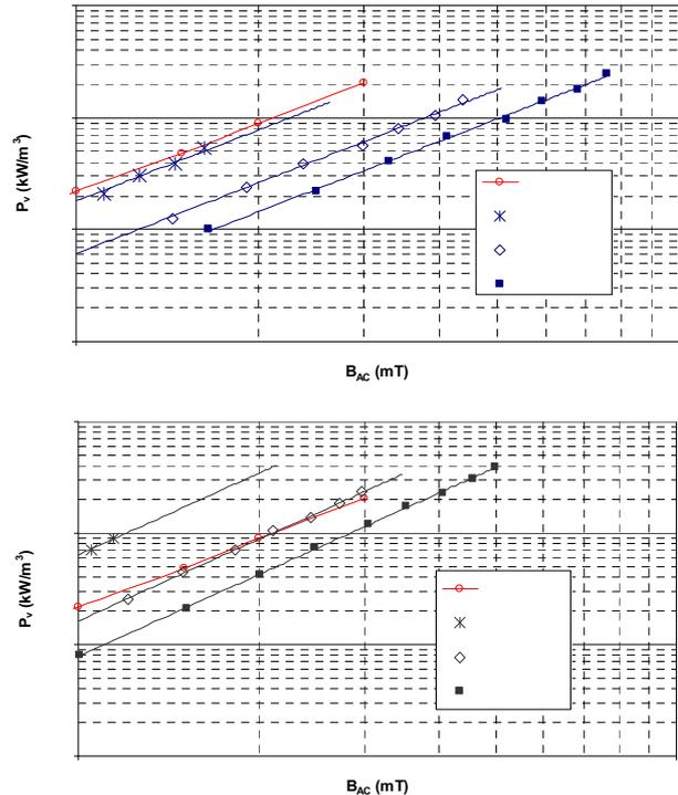
Fig. 6 Average power loss density vs average  $B_{AC}$  for (a) Alloy 1 and (b) Alloy 2
