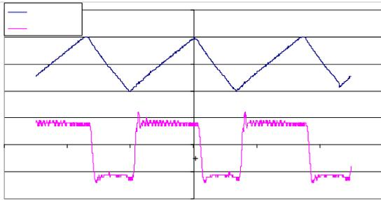
Fig. 11 Inductor voltage and current waveforms under 3 MHz DC/DC excitation
