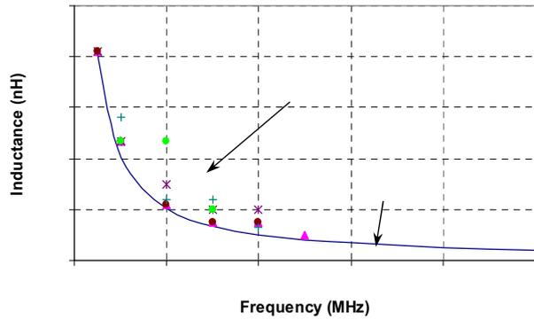
Fig. 2 Inductance vs. frequency for a 6 A POL supply
