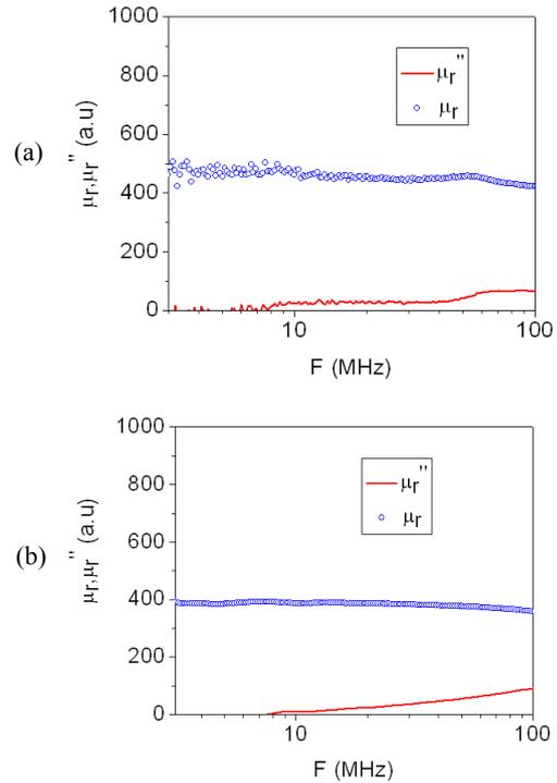
Fig. 4 Complex permeability of (a) Alloy 1 and (b) Alloy 2
