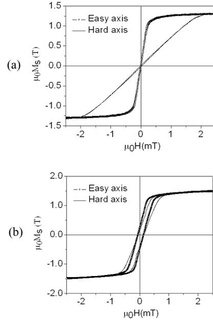
Fig. 3 BH loops of (a) Alloy 1 and (b) Alloy 2
