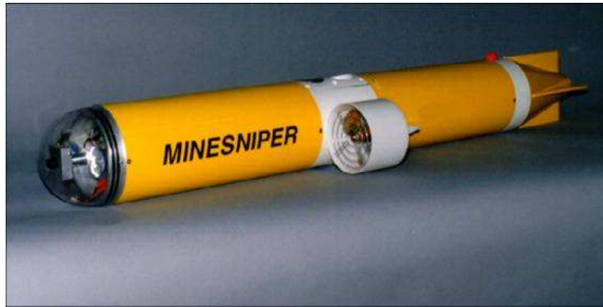
Figure 7.1: The Minesniper MK II, courtesy of Kongsberg ASA
