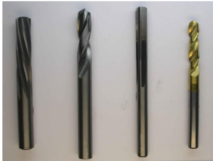
Figure 4 Carbide Tooling for Hole Drilling, Left to Right: Spiral Reamer, Drill, Straight Reamer, Tin Coated Carbide Drill.
