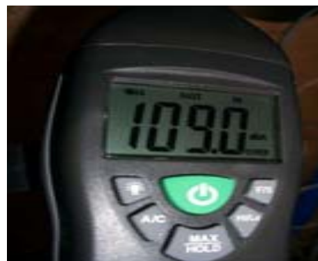
Figure 12 Measured SPL for the given pipe
