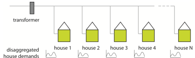
Figure 1. A row of houses being fed by a transformer.
