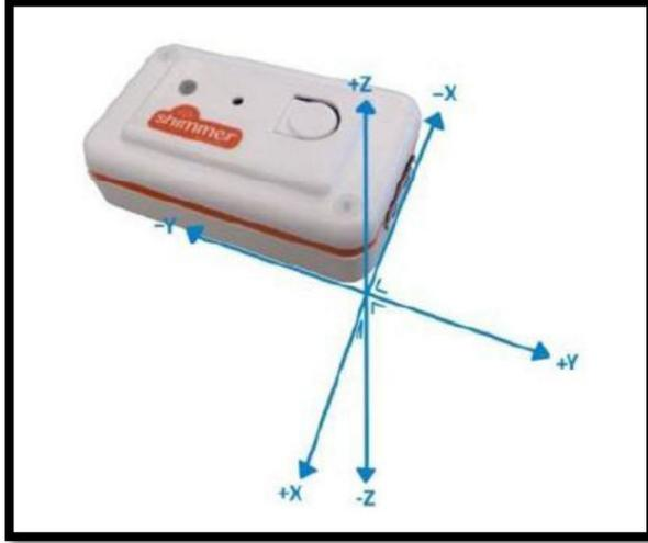
Figure 2: Accelerometer Coordinate System
