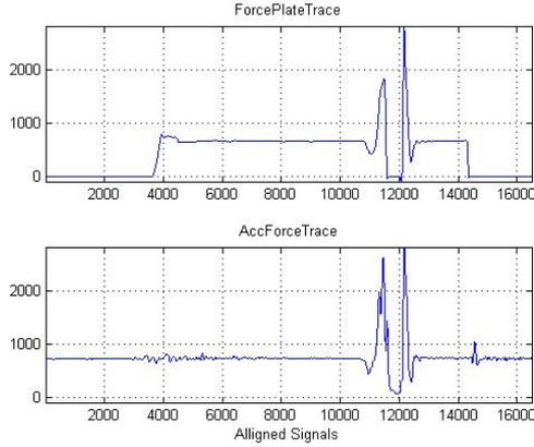
Figure 4: Aligned Force Platform and Accelerometer Trace
