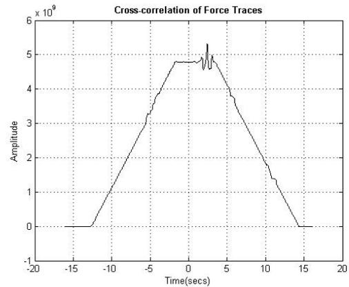
Figure 3: Cross Correlation of the Force Platform and Accelerometer Traces
