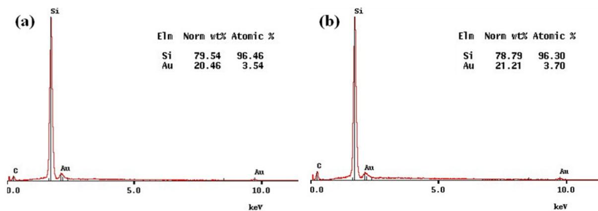
**Fig. 4.** XPS spectrum analysis of the PS samples (a) and (b) before immersion into SBF
