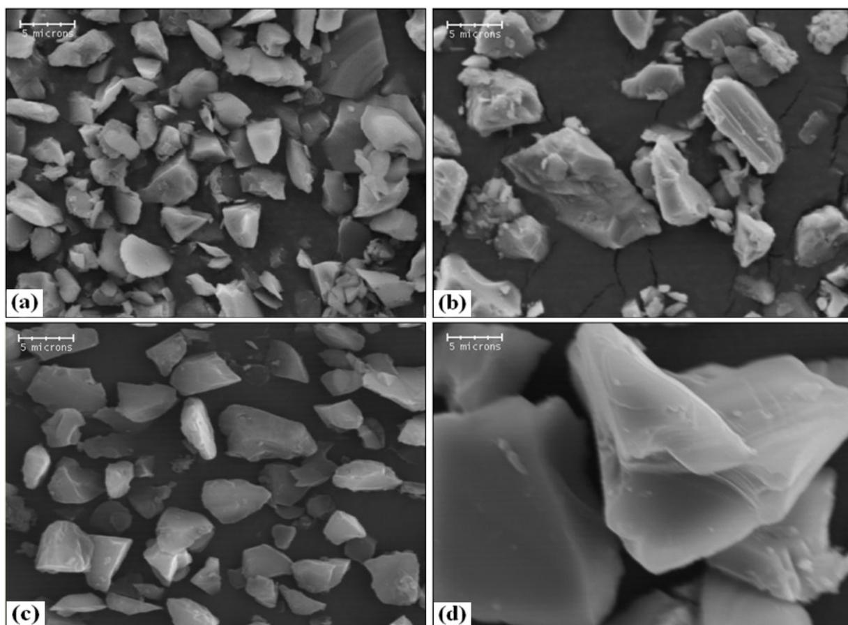
**Fig. 3.** SEM-EDX analysis of the PS samples (a) and (b) before immersion into SBF
