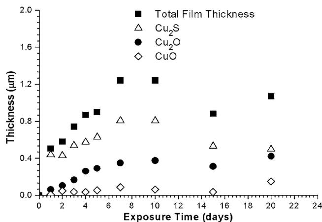
**Figure 4.** Calculated variation of corrosion layer thickness from cathodic reduction of Cu during exposure to class III MFG.
