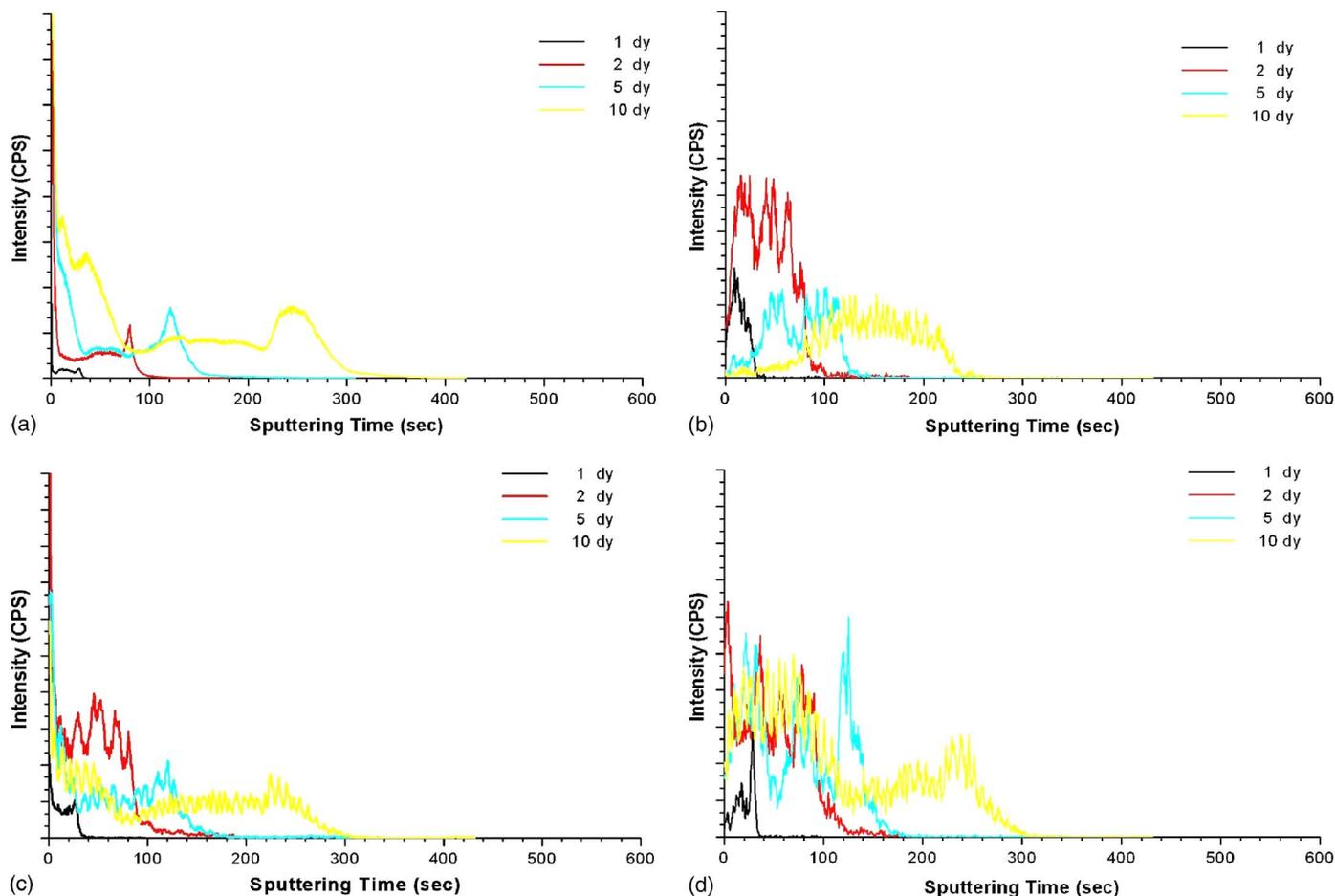
**Figure 10.** (Color online) SIMS depth profile of (a) Cu, (b) O, (c) S, and (d) Cl after 1, 2, 5, and 10 days in class III MFG.
