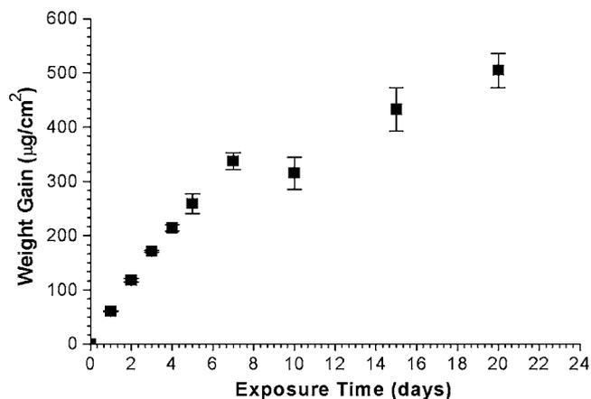
**Figure 2.** Mass gain vs time for Cu exposed to class III MFG.
