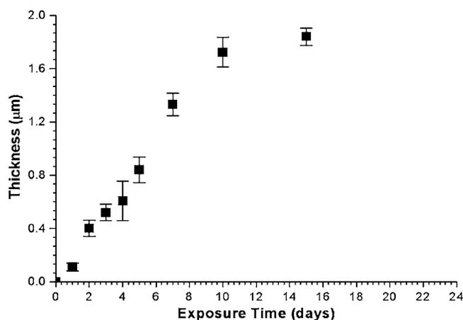
**Figure 8.** FIB cross-section measurements of corrosion layer thickness of Cu during exposure to class III MFG.
