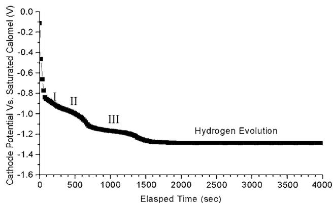
**Figure 3.** Cathodic reduction curve for Cu exposed for 2 day in class III MFG.
