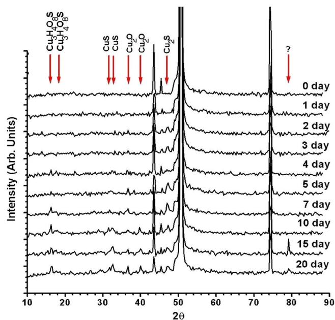
**Figure 5.** (Color online) X-ray diffractometer traces observed from Cu exposed for 0, 1, 2, 3, 4, 5, 7, 10, 15, and 20 days in class III MFG.
