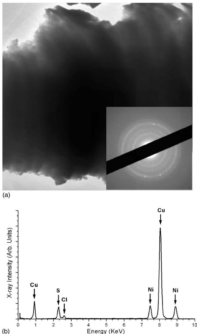
**Figure 6.** (a) TEM image with its corresponding SAED pattern. (b) EDS spectrum on corrosion product after 1 day class III MFG.
