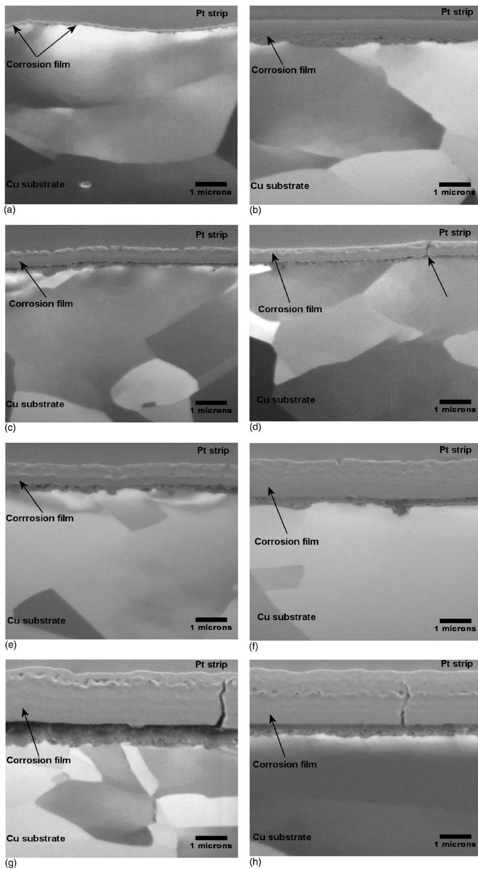
**Figure 7.** FIB-generated cross sections of Cu exposed to class III MFG for (a) 1, (b) 2, (c) 3, (d) 4, (e) 5, (f) 7, (g) 10, and (h) 15 days.
