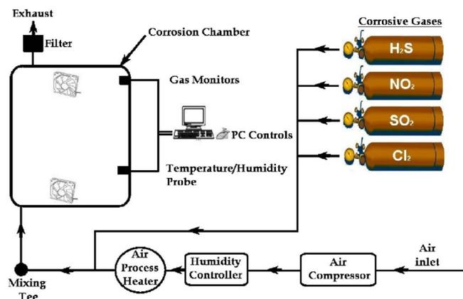
**Figure 1.** (Color online) Schematic diagram of the MFG test chamber setup.
