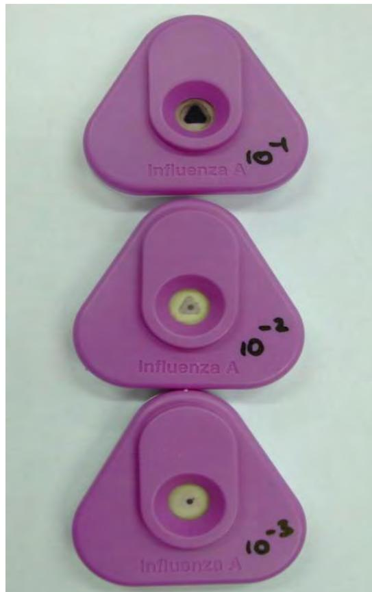
**Figure 2. 1 Directigen Flu A test cassettes following incubation with cultured EI virus A/eq/Kildare/89 at 3 dilutions ( $10^{-1}$ ,  $10^{-2}$  and  $10^{-3}$ )**
