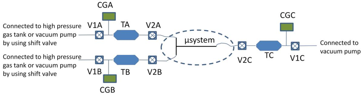
Figure1: Schema of test bench for gas mass flow rate measurement in T channel
