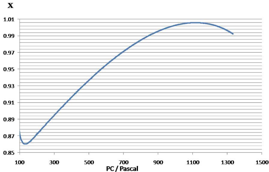
Figure 5: Ratio of mass flow rate measurement in TA and TB
