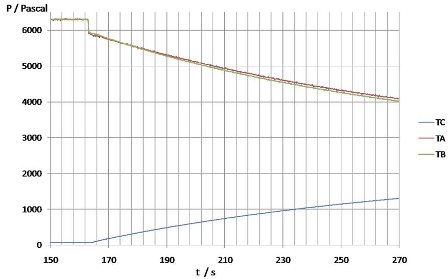
Figure 3: Pressure variation in TA, TB and TC during N<sub>2</sub> mass flow rate measurement
