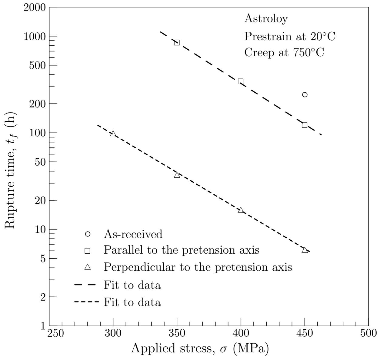
Figure 19: Time to fracture against effective stress for tensile creep tests of Astroloy (Adapted from [22]).
