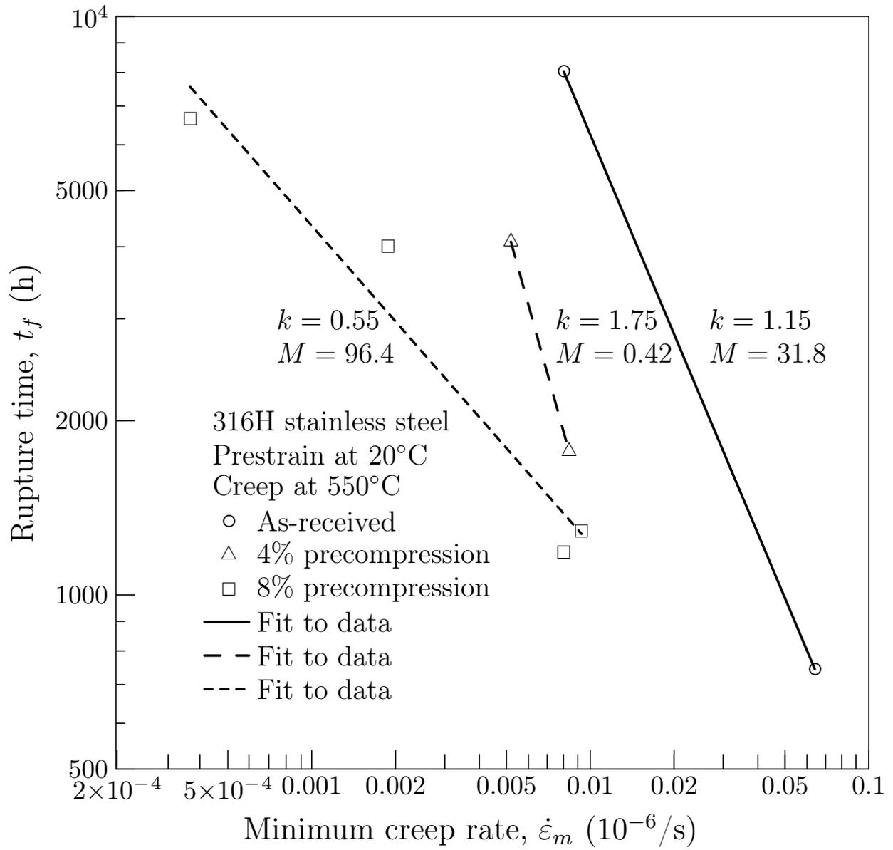
Figure 17: Precompression effects on high temperature (550°C) creep fracture behavior for 316H stainless steel (Data from [11]).
