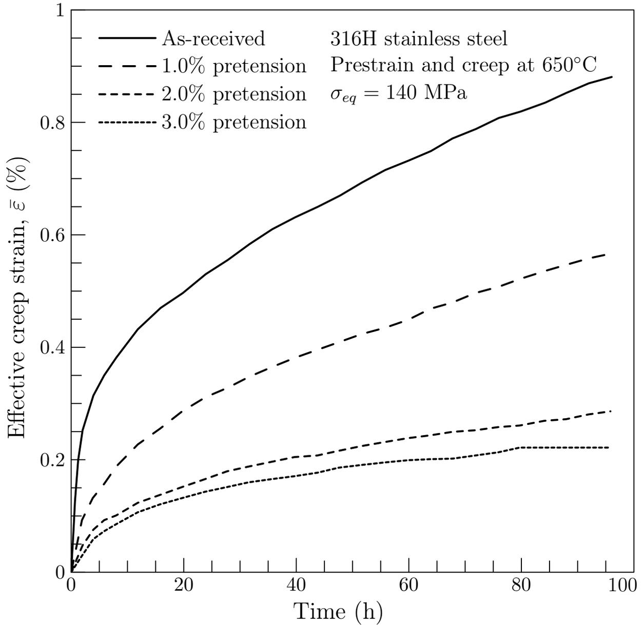
Figure 2: Effect of pretension on creep of 316H stainless steel under torsional loading (Adapted from [4]).
