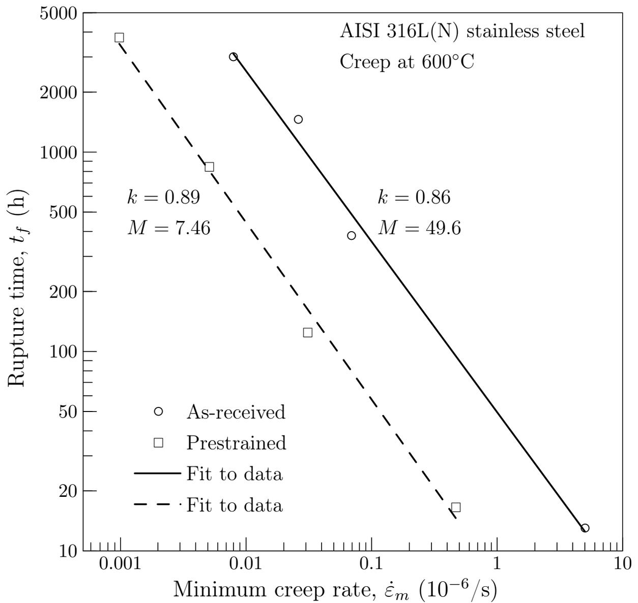
Figure 16: Prestraining effects on high temperature (600°C) creep fracture behavior for smooth cylindrical specimens (Data from [21]).
