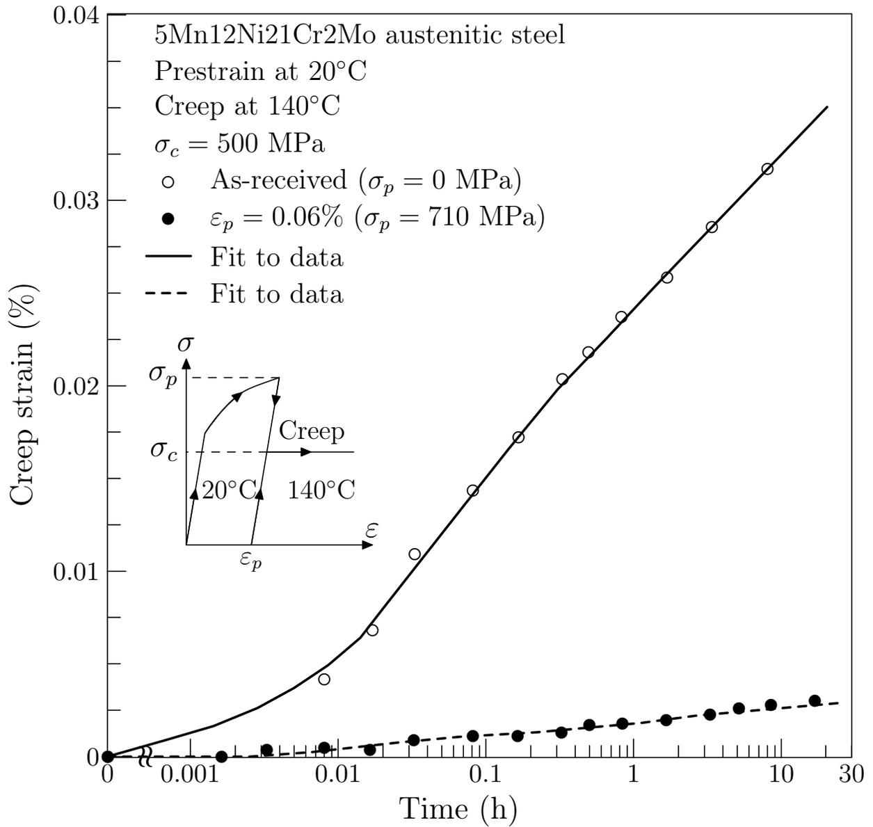
Figure 5: Room temperature prestraining effect on creep response of 5Mn12Ni21Cr2Mo austenitic steel at 500 MPa and 140°C (Adapted from [6]).
