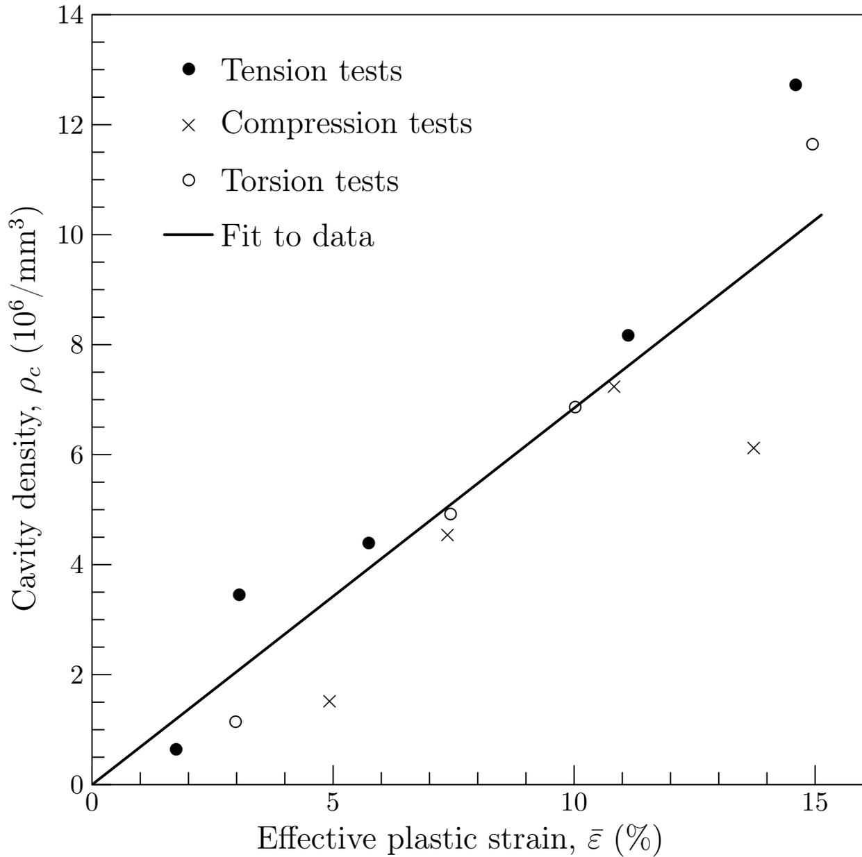
Figure 21: Variation of number of cavities per unit volume with effective plastic strain (Adapted from [14]).
