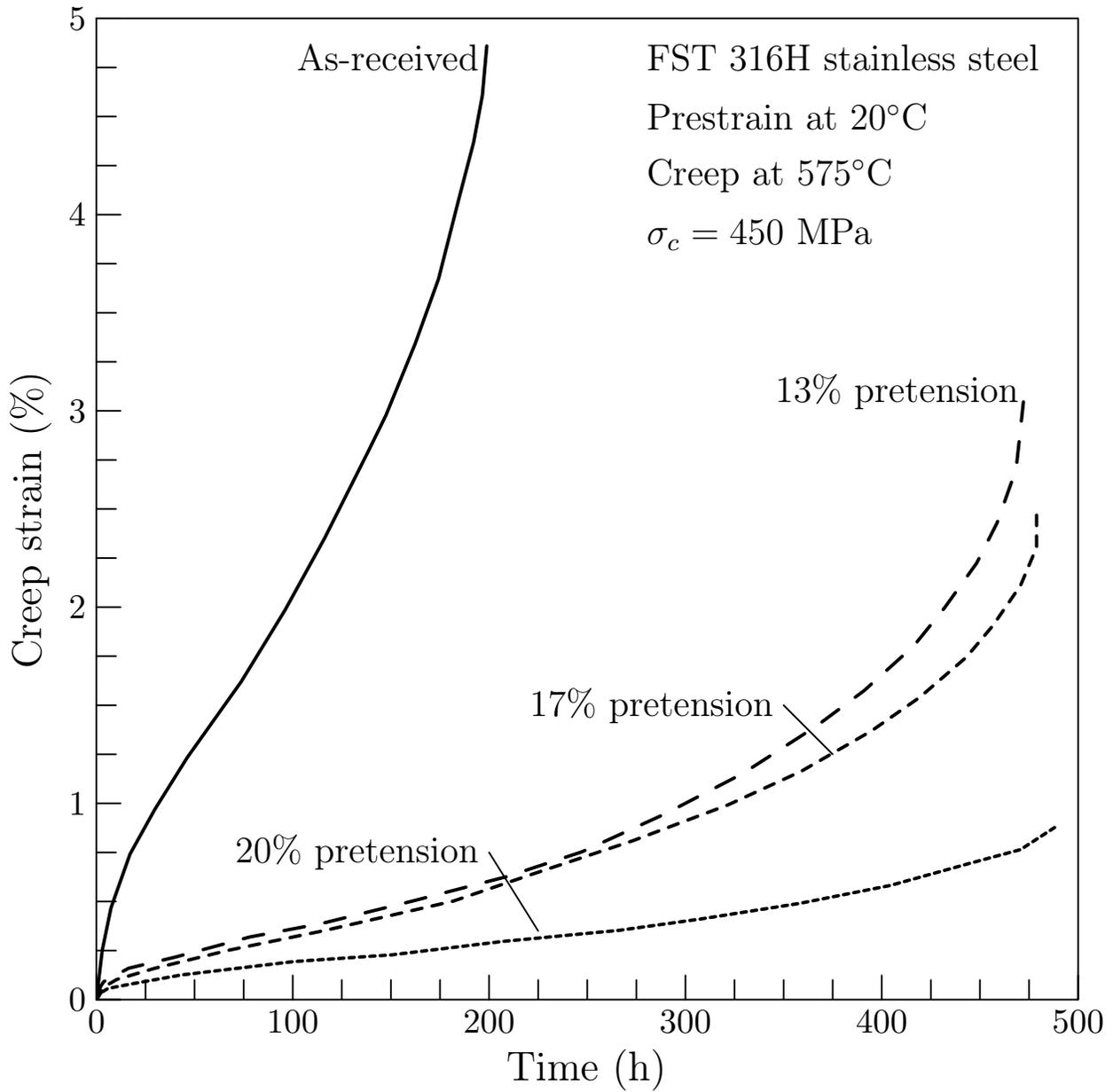
Figure 7: Creep responses at 450 MPa and 575°C of FST 316H stainless steel with different room temperature prestrains (Adapted from [2]).
