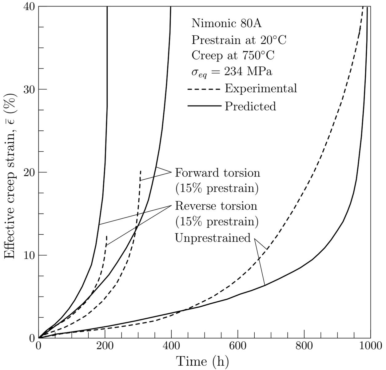
Figure 22: Torsion creep curves after pretorsion at room temperature for Nimonic 80A at 750°C where experimental and predicted curves are adapted from [14] and [33], respectively.
