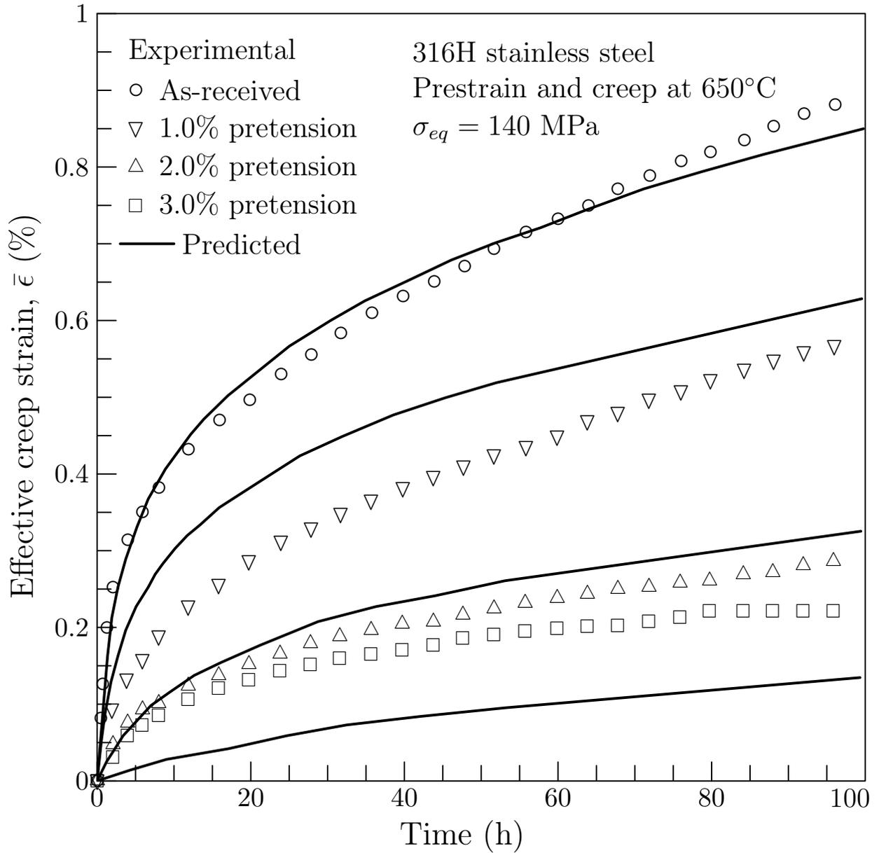
Figure 23: Torsion creep curves after pretension at 650°C for 316H stainless steel where experimental data and predicted curves are adapted from [4] and [35], respectively.
