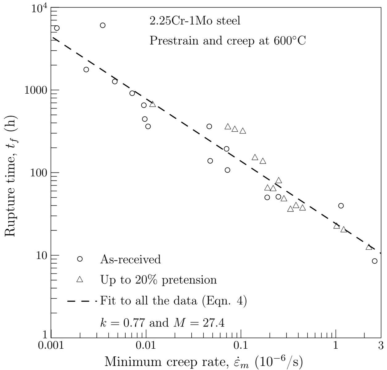
Figure 13: Monkman-Grant relation incorporating as-received and prestrained 2.25Cr-1Mo steels (Adapted from [13]).
