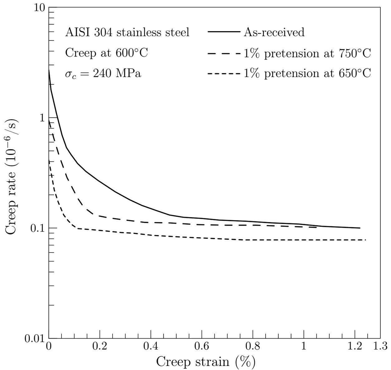
Figure 4: Effect of prestrain at various temperatures for 304 stainless steel (Adapted from [5]).
