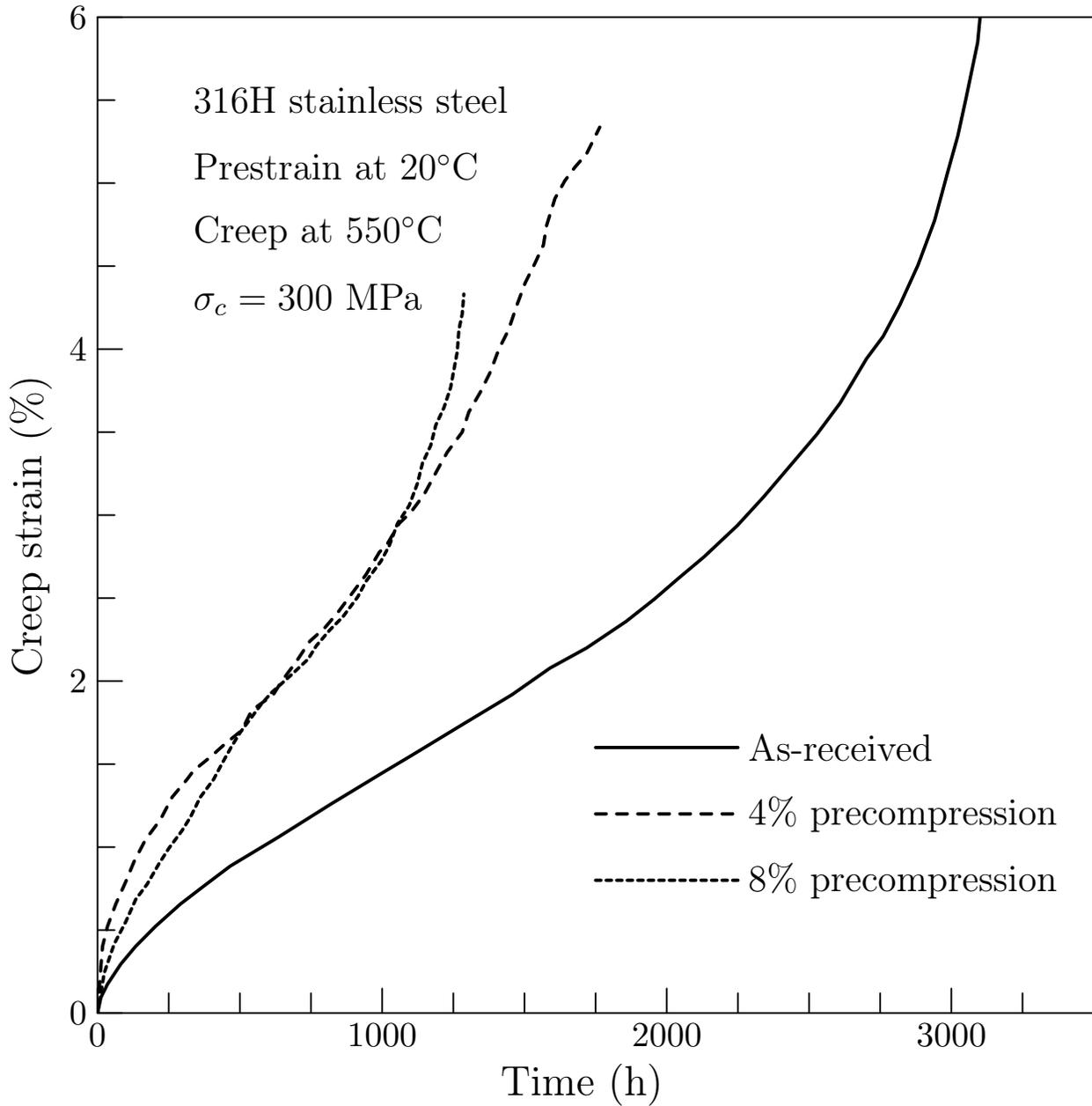
Figure 9: Creep curves at 550°C and 300 MPa for 316H stainless steel as-received and after prior deformation by 4% and 8% compression at room temperature (Adapted from [11]).
