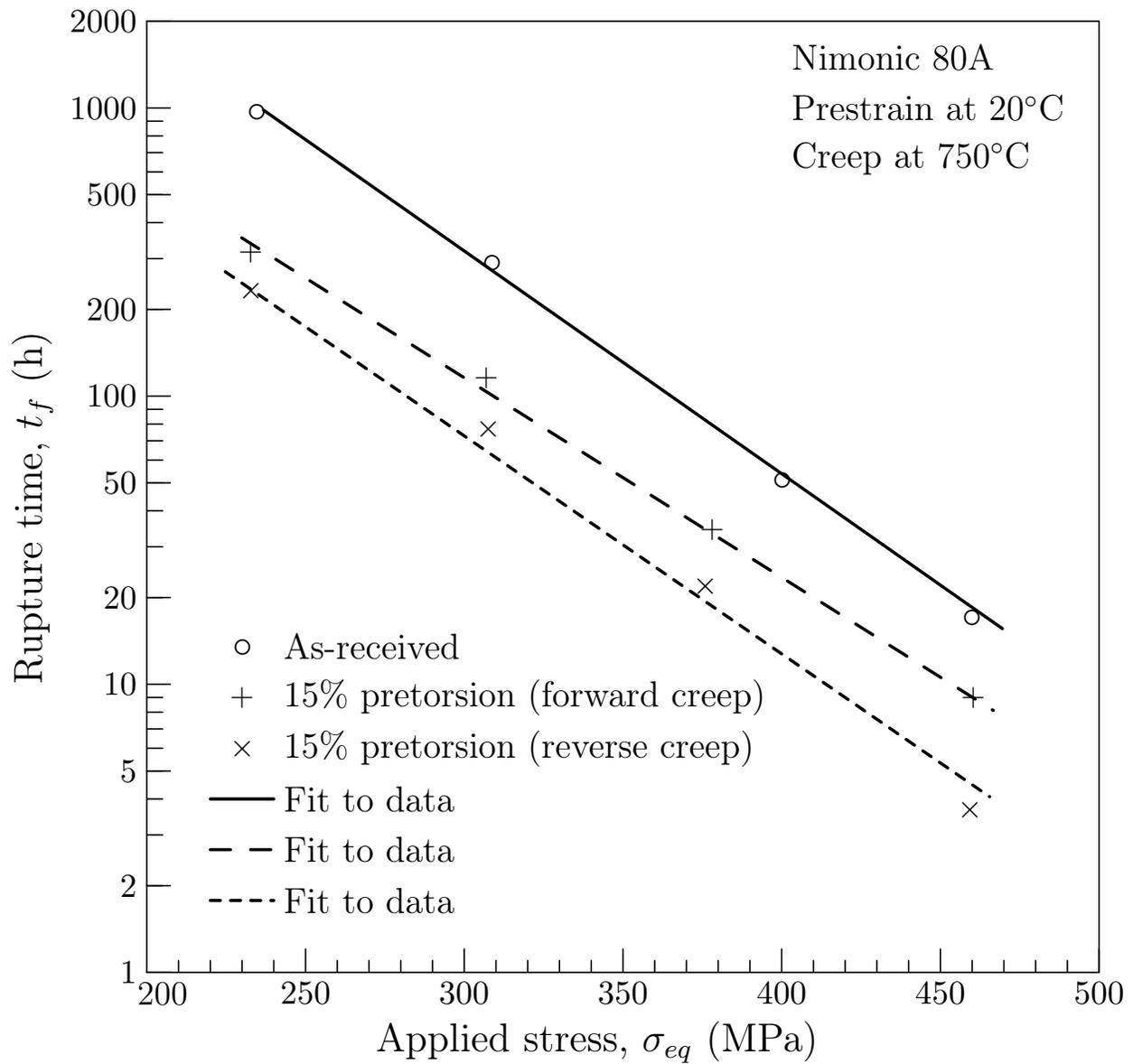
Figure 18: Time to fracture against effective stress for torsion creep tests of Nimonic 80A (Adapted from [14]).
