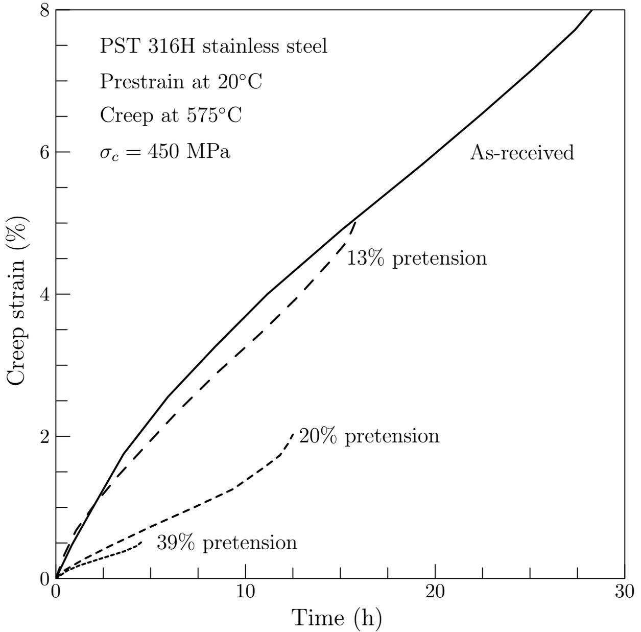
Figure 6: Creep responses at 450 MPa and 575°C of PST 316H stainless steel with different room temperature prestrains (Adapted from [2]).
