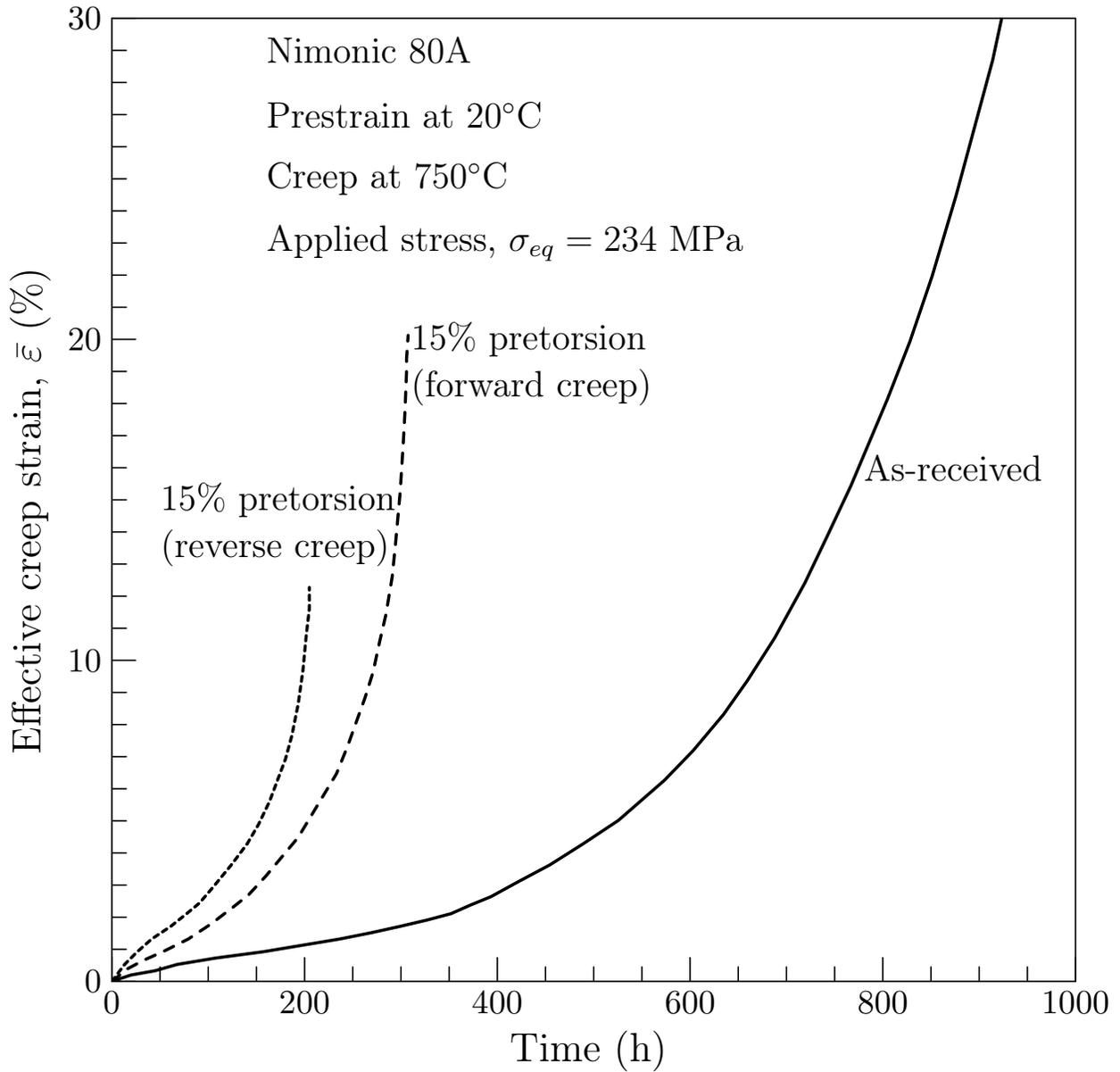
Figure 11: Torsion creep curves at 750°C and a equivalent stress of 300 MPa for Nimonic 80A (Adapted from [14]).
