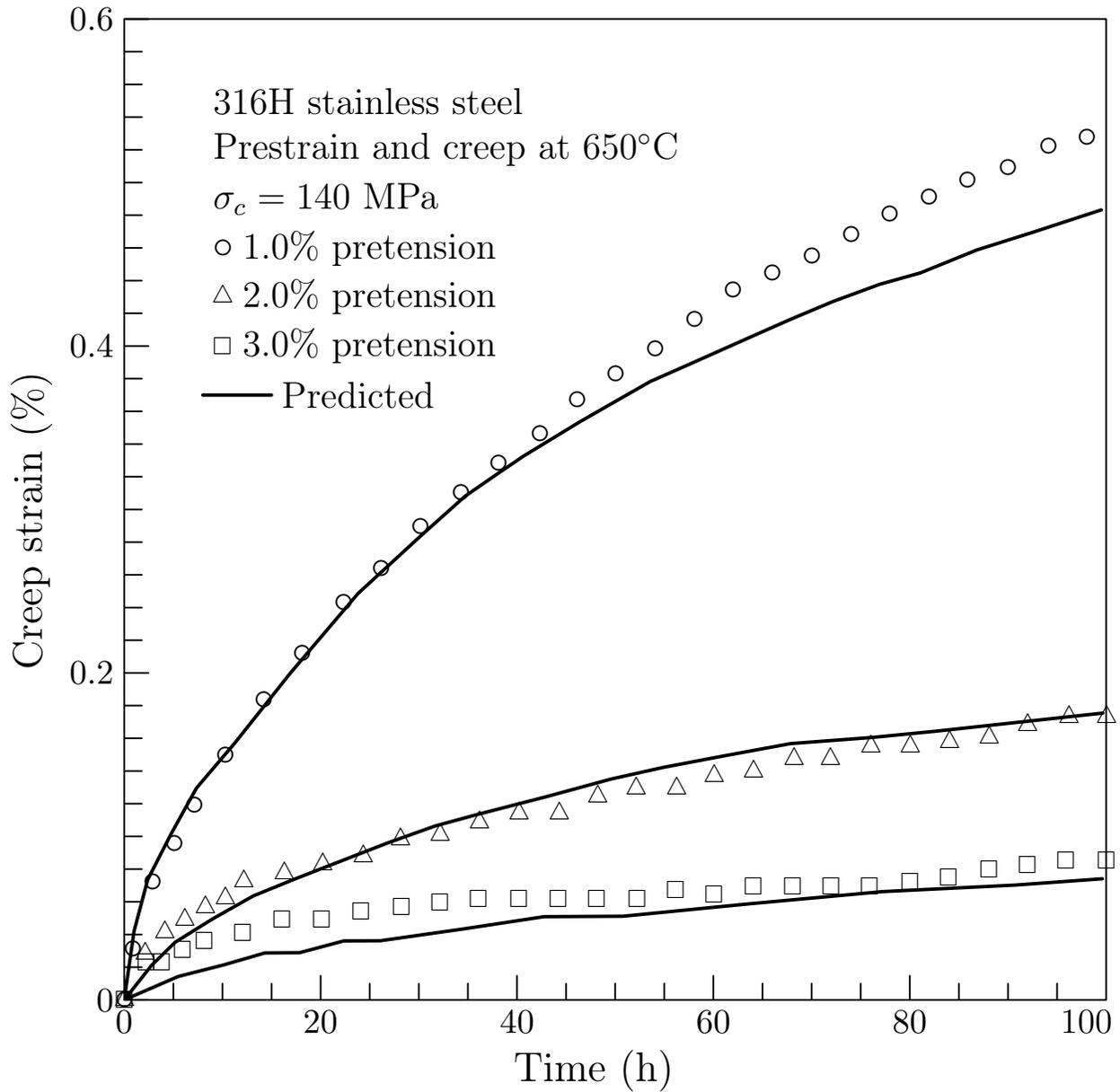
Figure 24: Tensile creep curves after pretension at 650°C for 316H stainless steel where experimental data and predicted curves are adapted from [4] and [36], respectively.
