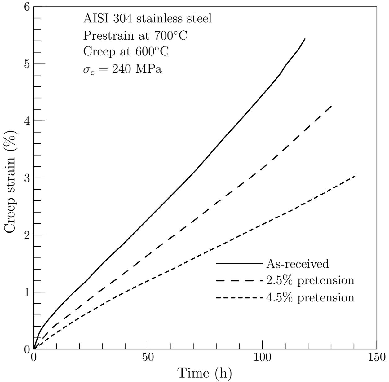
Figure 3: Prestraining results in [5] for 304 stainless steel (Adapted from [5]).
