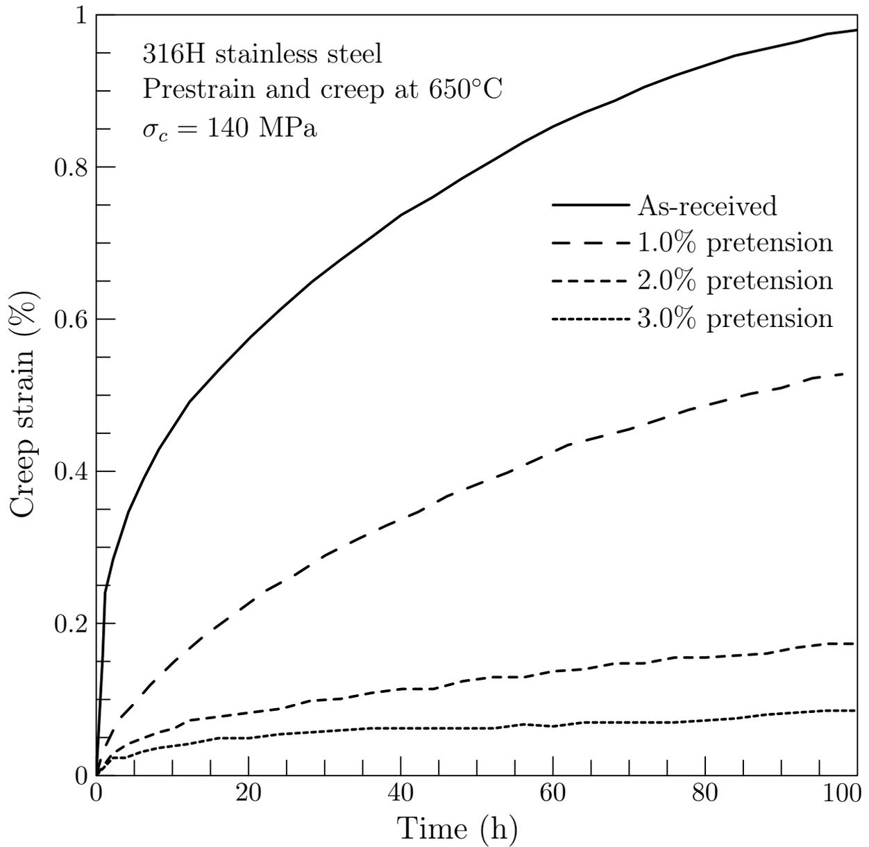
Figure 1: Effect of prestrain on creep of 316H stainless steel under uniaxial tension (Adapted from [4]).
