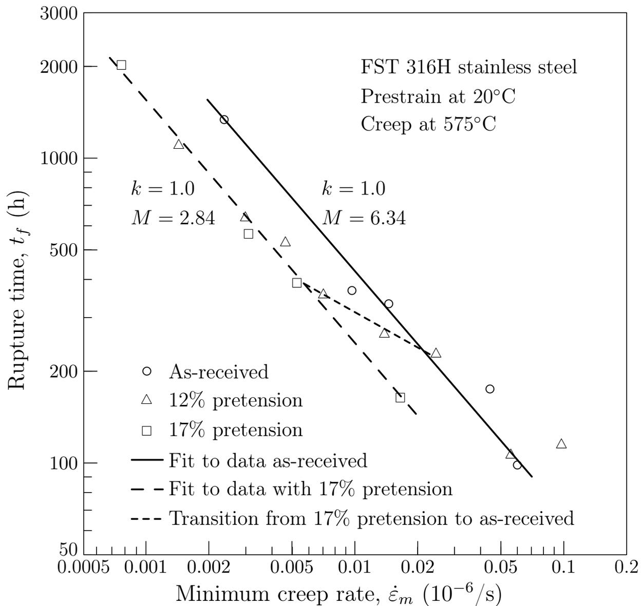
Figure 15: Monkman-Grant relation incorporating as-received and prestrained FST 316H stainless steels (Adapted from [2]).
