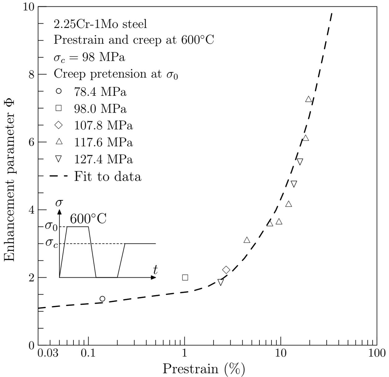
Figure 10: Creep enhancement as a function of amount of prestrain in creep test of 2.25Cr-1Mo ferritic steel at 600°C (Adapted from [13]).
