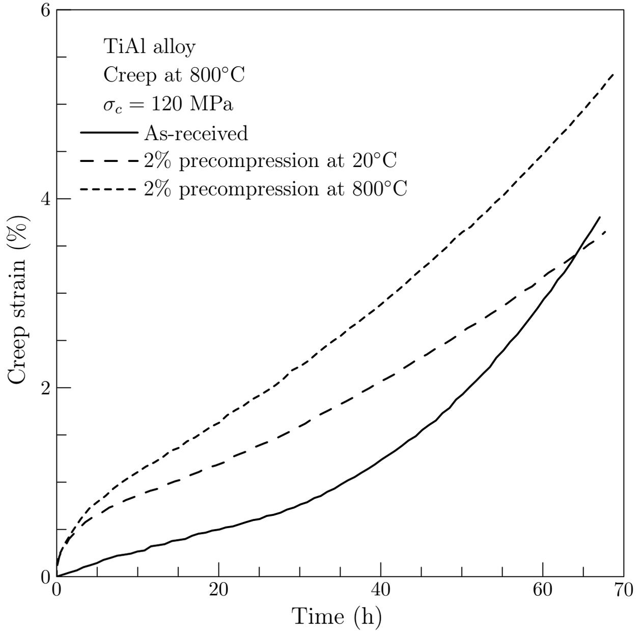
Figure 12: Creep curves at 800°C and 120 MPa for polycrystalline TiAl alloy as-received and after prior deformation by 2% at room temperature and 800°C (Adapted from [17]).
