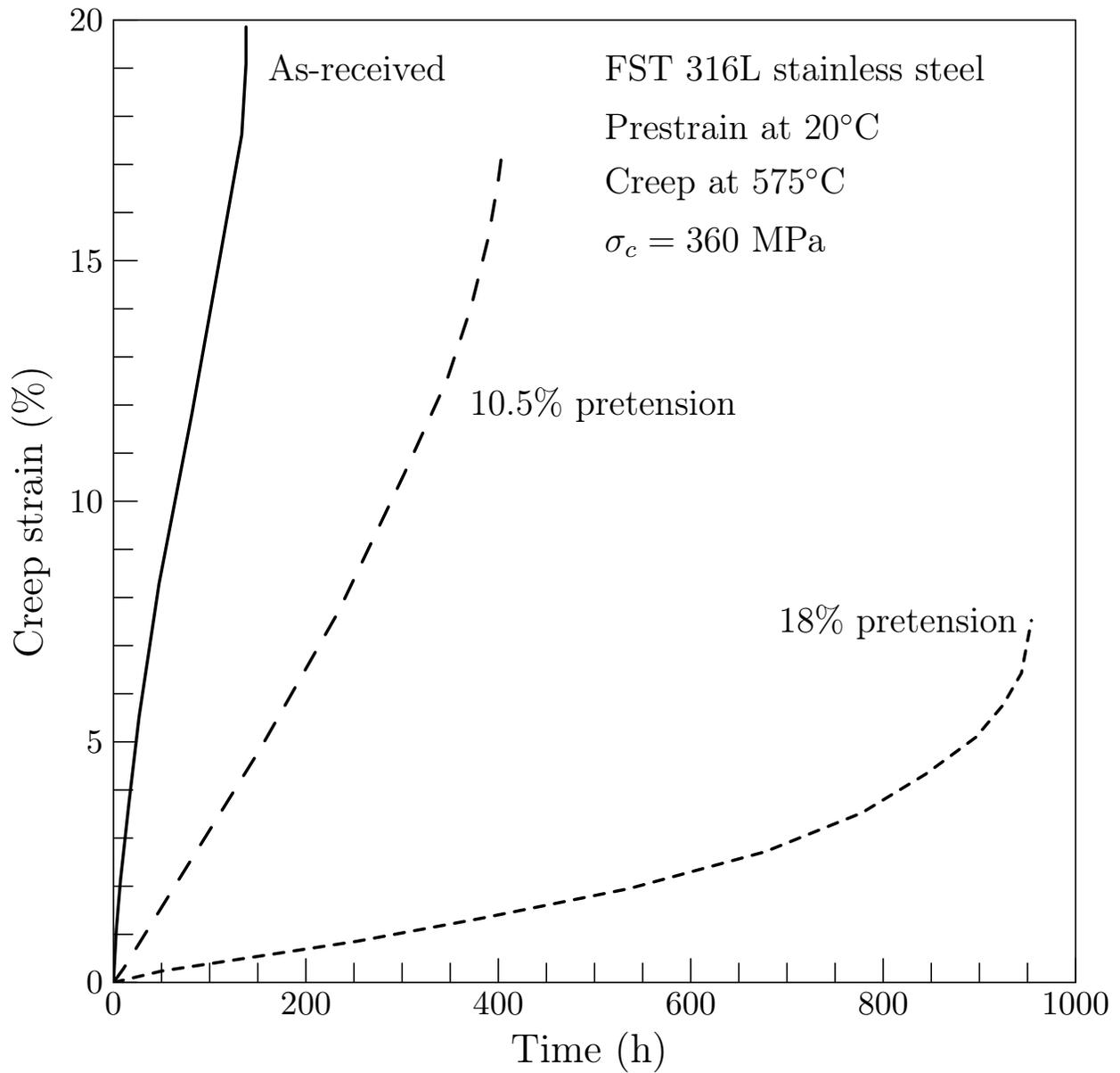
Figure 8: Creep responses at 360 MPa and 575°C of FST 316L stainless steel with different room temperature prestrains (Adapted from [2]).
