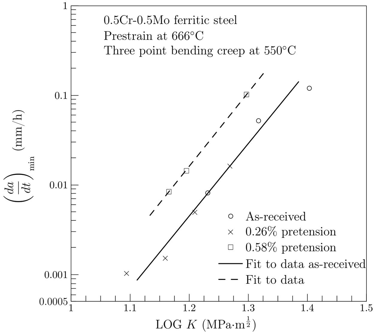
Figure 20: High temperature pretension effects on the subsequent creep crack growth. (Adapted from [23]).
