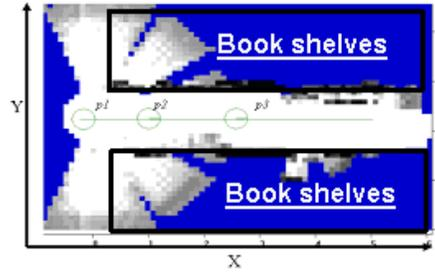
**Fig. 6. Sonar readings as robot traverses aisle**
