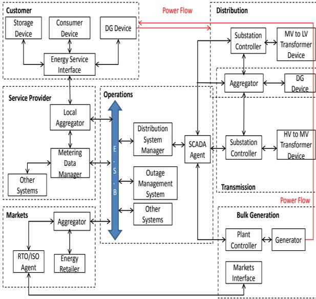
Figure 2. Reference Software Architecture for the Smart Grid
