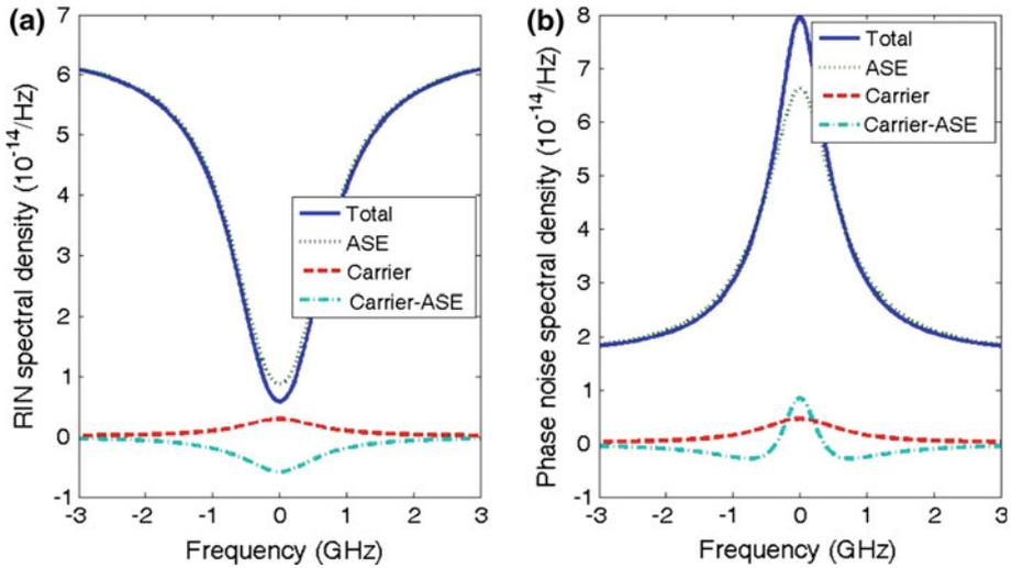
**Fig. 2** SOA booster output, **a** total RIN and its components spectra, **b** total phase noise and its components spectra. The spectra are centered at the input optical frequency. The normalised input power is 0.1
