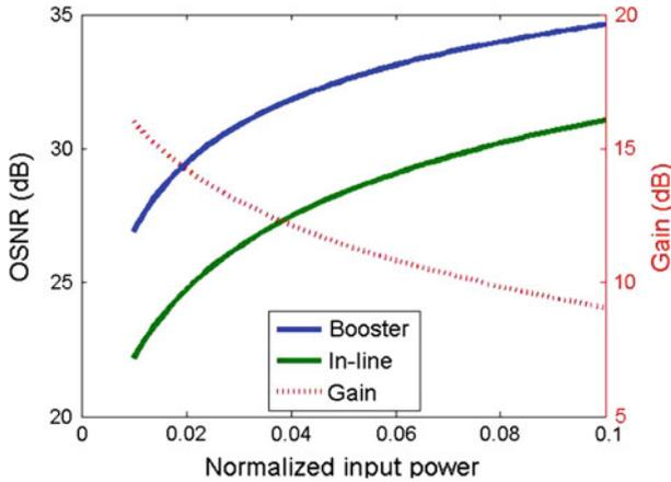
Fig. 6 OSNR versus normalized input power for the booster and in-line amplifiers
