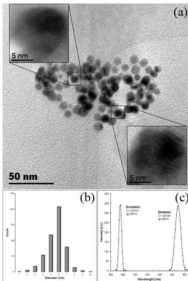
**Fig. 1** (a) Low and high resolution TEM images of an area of silicon nanocrystals synthesised with ODPa and (b) the corresponding particle size distribution histogram. Room temperature photoluminescence spectrum with excitation at 335 nm and the corresponding emission peak at 450 nm (c).
