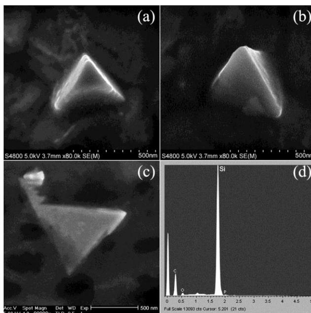
**Fig. 6** HRSEM images (a,b) of well faceted silicon tetrahedra, synthesized from a TOP/sc-CO<sub>2</sub> system. SEM image (c) of silicon tetrahedra with corresponding EDX spectrum (d).
