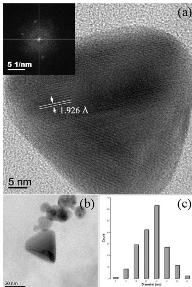
**Fig. 2** HRTEM image of a truncated tetrahedral-shaped nanocrystal with corresponding fast Fourier transform inset (a). TEM image of a mixture of truncated nanotetrahedra and pseudo spherical nanocrystals synthesized using DDPA (b) with the corresponding particle size distribution histogram (c).
