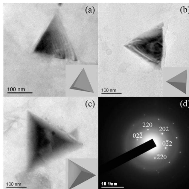
**Fig. 5** TEM images of silicon tetrahedra with inset CAD models, portraying their geometrical orientation (a-c). A single crystal pattern (d), from the selective area electron diffraction analysis of (c).
