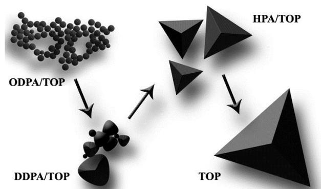
**Fig. 8** A schematic showing the effect of the phosphonic acid on the size and shape evolution of pseudo-spherical silicon nanocrystals to larger truncated nanotetrahedra and finally to fully formed silicon tetrahedral-shaped crystals.
