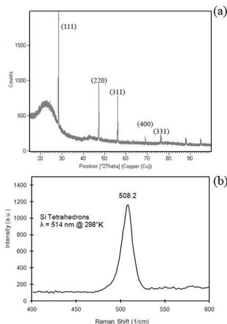
**Fig. 7** An example of a XRD spectrum collected from as-synthesized black powders (a). The XRD pattern indexes to diamond cubic Si and also shows a broad peak at the beginning which can be attributed to silicon oxide by-products. Raman spectrum of TOP capped silicon tetrahedra (b).
