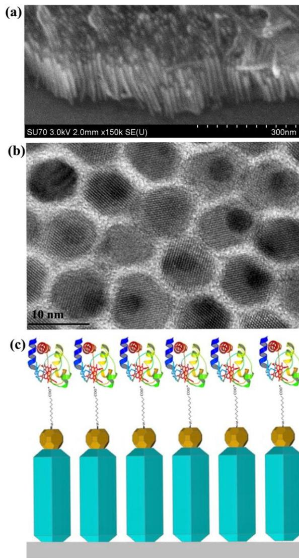
**Fig. 1.** Side view HRSEM image of (a) perpendicularly aligned nanorods (b) HRTEM top down image of gold tipped nanorods (c) schematic showing the bottom up assembly process consisting of gold tipped nanorods on an ITO substrate
