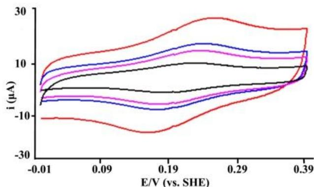
**Fig. 2.** Cyclic voltammogram (C.V) of cyt c immobilisation via HS(CH<sub>2</sub>)<sub>10</sub>COOH/HS(CH<sub>2</sub>)<sub>7</sub>OH onto gold tipped nanorods in 10 mM phosphate buffer, pH 7.4 at 20 mVs<sup>-1</sup> (—), 40 mVs<sup>-1</sup> (—), 50 mVs<sup>-1</sup> (—) and 100 mV s<sup>-1</sup> (—).
