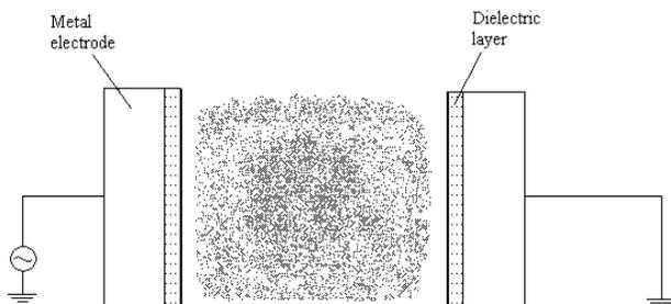
Figure 1: Dielectric barrier discharge plasma system
